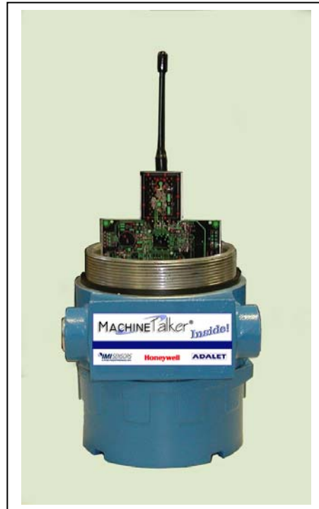
Talker® Model CBM6 - Includes High-Speed A/D Converters and Power Switches for programmed turning on of sensors. Shown Mounted Inside Explosion-Proof Enclosure for gaseous environments.
